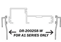
Flange can be installed on either side to provide either inswing or outswing application
